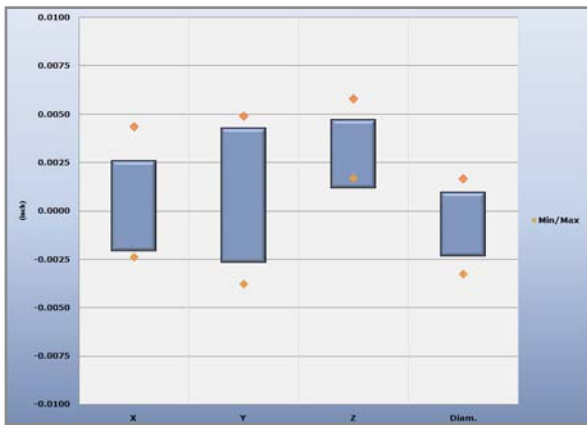
Figure 9: Plot of dimensional deviations (two sigma) by measurement axis. Results for cylindrical measurements in the XY-plane are also listed.
