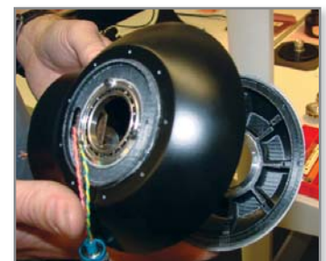
Direct digital manufacturing: FDM is used to produce 20 of the COLIBRI’s components, including the enclosure.
