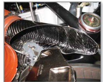
The new outlet was bolted onto the car in time for the next race -- only three days after the overheating problem.
