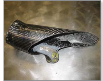
Wednesday: Final air-duct outlet is produced from carbon fiber composite.
