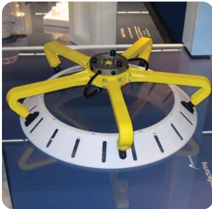
Image 1: Components for this robotic gripper were first prototyped, then manufactured, using FDM (Fused Deposition Modeling). Image 2: The robot is used by an injection molder to hold and transfer large, conical parts.
