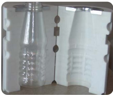
Figure 12: To mold the PET bottle, this hybrid insert uses a cylindrical design.
