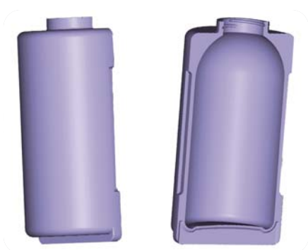
Figure 11: CAD data for a contoured insert that is mounted in a machined mold base.
