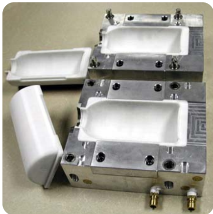
Figure 10: FDM hybrid tool with contoured inserts.
