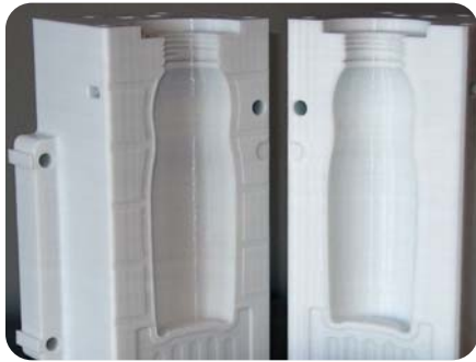
Figure 9: FDM blow molding tool made from polycarbonate.
