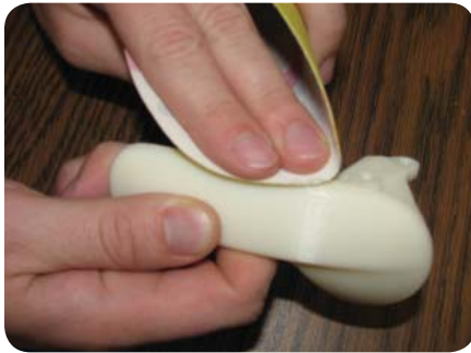
Figure 4: Sanding. Using appropriate grit sandpaper, remove FDM build layer lines.
