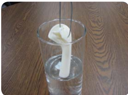
Figure 6: Sealing. Seal the part's surfaces by dipping in solvent.
