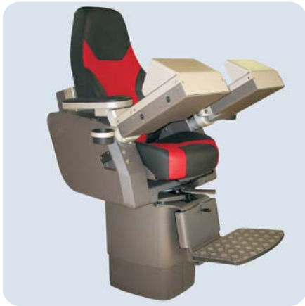
Images 1 and 2: Designed for an offshore oil-drilling rig, this drill-operator control chair was prototyped with the help of an FDM Vantage. Then 25 of its components were manufactured by the same Vantage.
