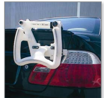
In the jigs and fixtures department at BMW AG, Regensburg, a Fortus system is used to manufacture assembly tools. This tool is used to affix the rear name badge.
