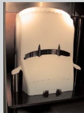
Figure 7: 1/4 scale part built on FDM Maxum
