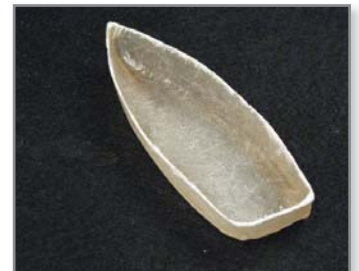
Finished Fiberglass part using an FDM mold.
