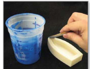
Figure 3: The epoxy is uniformly applied to all surfaces that will have contact with the fiberglass resin.
