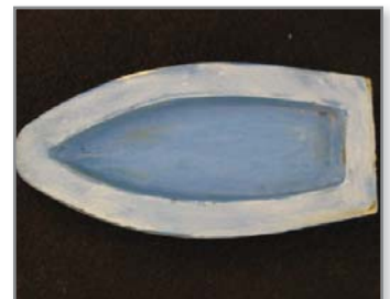
Figure 4: After the epoxy has cured, the mold surface is sanded and buffed to the desired finish.
