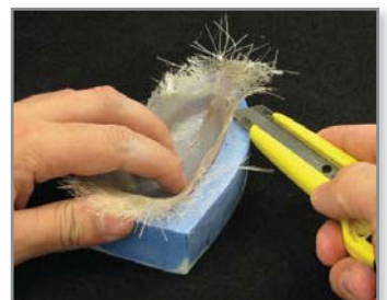
Figure 5: After the lay-up process, the part is trimmed and removed from the mold.
