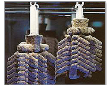
Figure 5: Parts on casting tree after shelling process.
