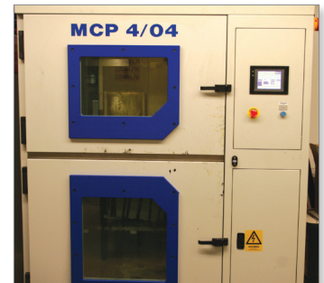
Figure 8: The two-part urethane and RTV mold are placed in the automated vacuum casting machine.
