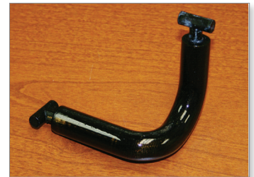
Figure 4: A soluble core for the radiator hose.
