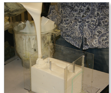
Figure 6: The RTV rubber is poured into the pattern and then allowed to cure.
