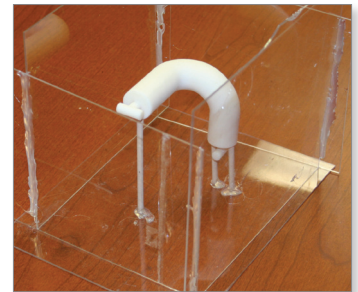
Figure 5: The pattern is mounted on dowels and attached to the floor of the mold box.
