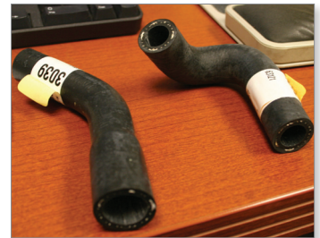
Figure 1: These hoses are examples of parts that need soluble cores since the RTV tool cannot be extracted from the internal passage.
