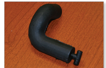
Figure 10: Finished hose part with soluble core in.
