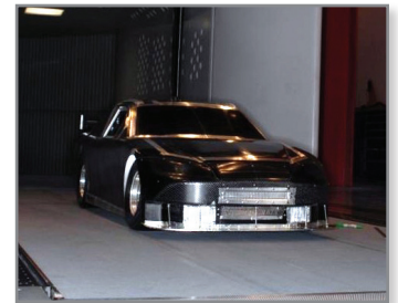
Figure 1: NASCAR teams rely on rolling-floor wind tunnels to analyze aerodynamics of their race cars.
